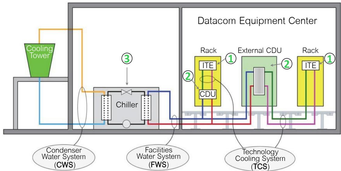
**Heat capture within the server** – This is achieved with either cold plates directly attached to components (i.e., GPUs) or with immersion cooling (not discussed in this paper since DLC is the prevalent means in the industry). Coolant flowing through the cold plates transports the heat energy out of the server and into the CDU.
